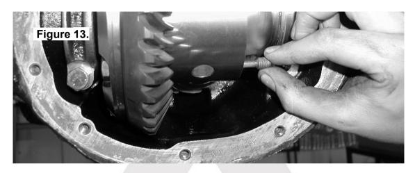
Completely remove the long cross shaft (Fig.14.).
