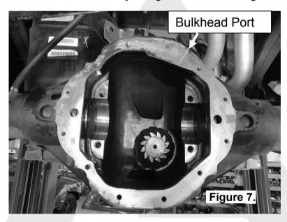
NOTE: It is a good idea to place a magnet on the inside of the differential housing to collect metal filings when drilling & tapping.
